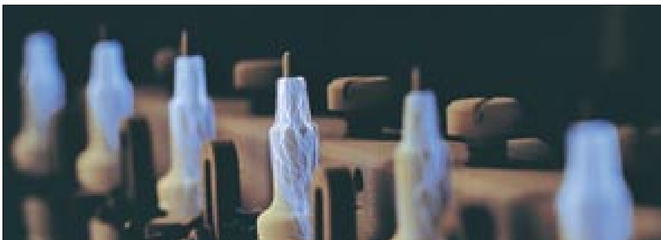
Testing an insulator at 40,000 Volts.
